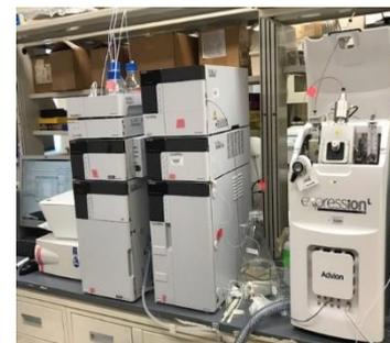
Advion Expression LC-MS (CMS-L01 model) with Shimadzu HPLC (LC20AB model)
